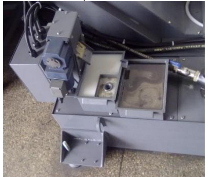
Oil separate system for coolant
